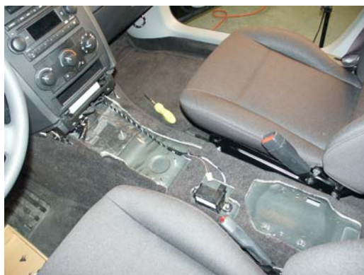
Remove OEM track/plate & plastic trim covering
